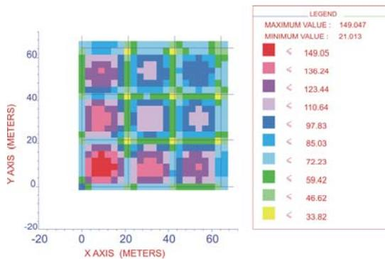
Figure 12. Touch Voltages over the Immersed Region of the Grid: Hemispherical Soil Volume.
