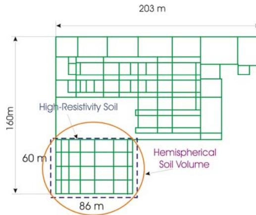
Figure 13. Grid Partially Immersed in High Resistivity Soil Volume.
