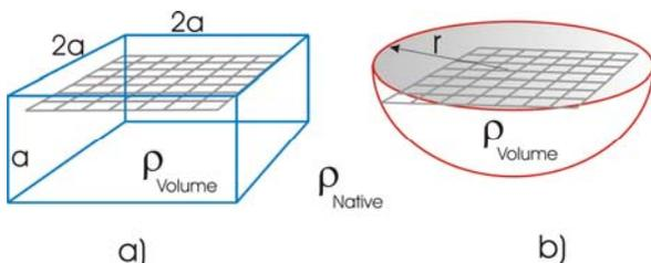
Figure 1. Rectangular (a) and Hemispherical (b) Soil Models.
