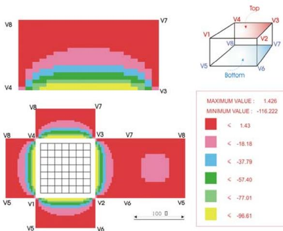
Figure 4. Charge Density Distribution over Rectangular Volume Surfaces:  $\rho_{Volume} \gg \rho_{Native}$  ( $\rho_{Volume}=1000 \Omega\text{-m}$  and  $\rho_{Native}=10 \Omega\text{-m}$ ).
