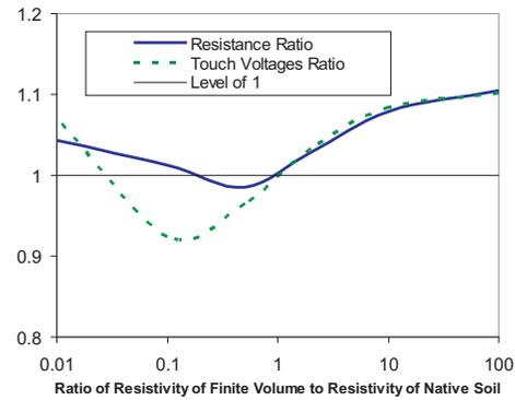
Figure 2. Resistance Ratio and Maximum Touch Voltage Ratio as a Function of Resistivity Ratio.
