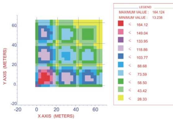
Figure 11. Touch Voltages over the Immersed Region of the Grid: Rectangular Soil Volume.
