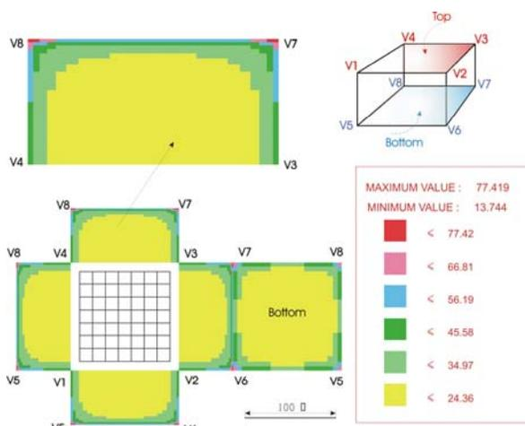
Figure 3. Charge Density Distribution over Rectangular Volume Surfaces:  $\rho_{Volume} \ll \rho_{Native}$  ( $\rho_{Volume}=10 \Omega\text{-m}$  and  $\rho_{Native}=1000 \Omega\text{-m}$ ).
