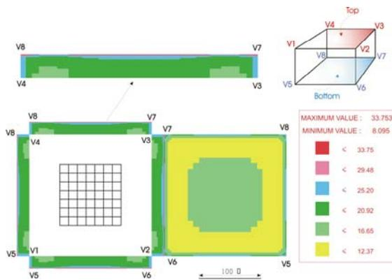
Figure 7. Charge Density Distribution over the Rectangular Volume Surfaces:  $\rho_1=200\Omega\text{-m}$  and  $\rho_2=1000\Omega\text{-m}$ . Volume Dimensions Are  $200\text{ms}\times 200\text{ms}\times 20\text{m}$ .
