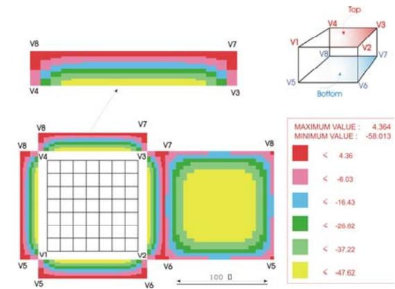
Figure 8. Charge Density Distribution over the Rectangular Volume Surfaces:  $\rho_1=1000\Omega\text{-m}$  and  $\rho_2=200\Omega\text{-m}$ . Volume Dimensions Are  $120\text{ms}\times 120\text{ms}\times 20\text{m}$ .
